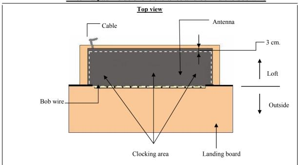
Attention! Install the antenna with the cable outside
