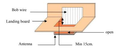
On the landing board, you can build an area which is lower. The antenna is installed under the area.
