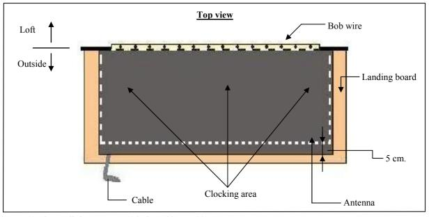
Attention! Install the antenna with the cable outside
