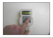
• The orange navigation keys <PREVIOUS> and <NEXT> allow you to scroll through the clocking-list. When a pigeon arrives the display automatically shows the latest clocking.
