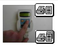
Printing: Through the menu on your Speedy, the are two printouts options - a complete overview-list or a clocking-list. To print, Speedy should be connected with a printer-interface. You can then use any DOS compatible printer.
