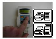
**Printing:** Trough the menu on your Speedy, 2 printouts are possible. A complete overview-list or a clocking-list. To print, Speedy is connected over a printer-interface. You can use all DOS compatible printers.
