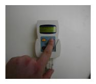
Connect the loft-antenna cable to the speedy. (the male cableend, with pins) Before connecting additional antennas they first need to be programmed (page 10)
