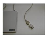
• After programming all loft-antennas, the installation can be completed by connecting all antennas to each other. Male plug into female plug. Assure yourself that there is a male plug pointing to the speedy. At the end of the installation, connect an endplug to close the circuit. With "antenna test" you can easily test the installation. (page 10)
